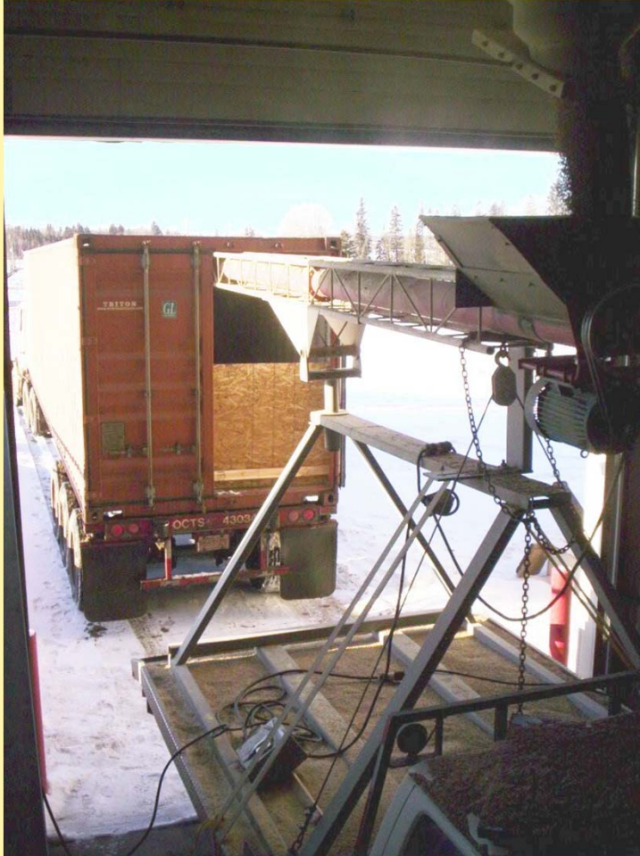
Mobile auger for loading from multiple bin locations throughout the facility.
