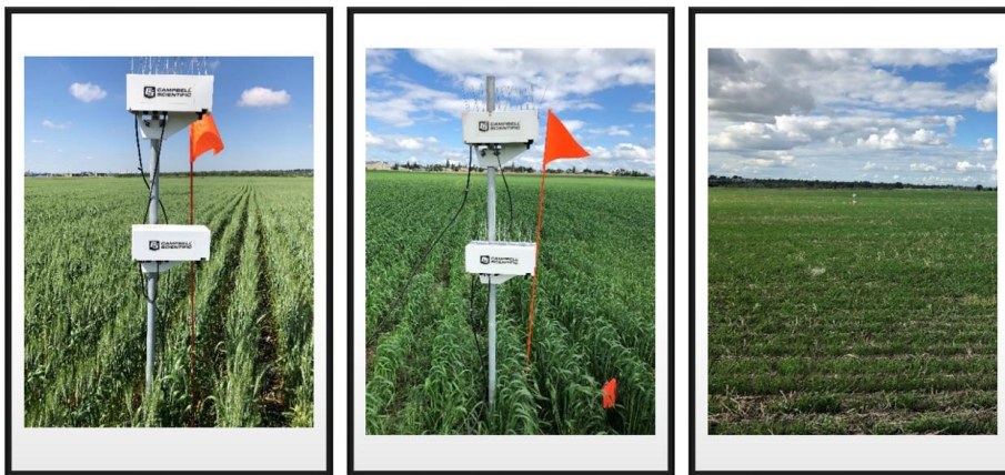
Photos of the micromet equipment (loggers, anemometer, and sampling towers) during canola production in 2021 (Photo credit: Kate Congreves)
