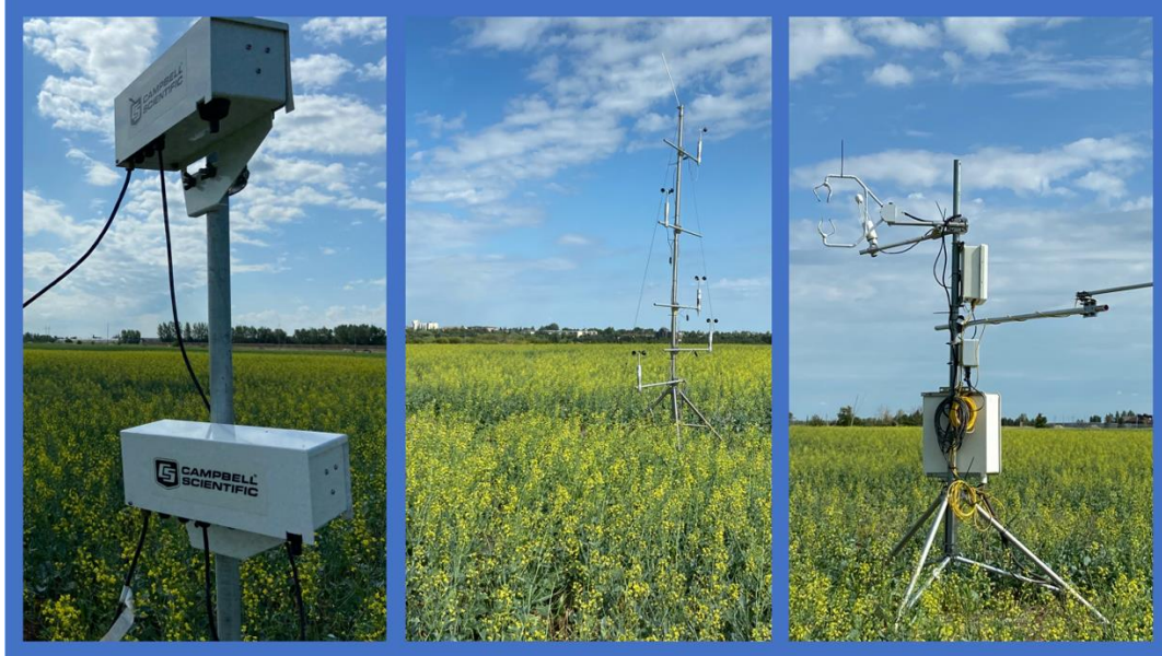
Figure 1 Photos of the micromet equipment (loggers, anemometer, and sampling towers) during canola production in 2021 (Photo credit: Kate Congreves).
